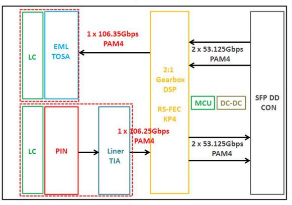
Figure 1. Module Block Diagram
