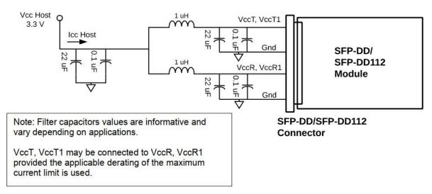
Figure 3. Host Board Power Supply Filtering
