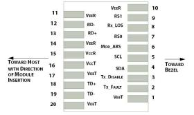
Figure 2. Electrical Pin-out Details
