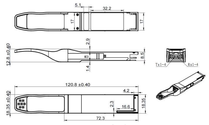
Figure 12. Mechanical Specifications
