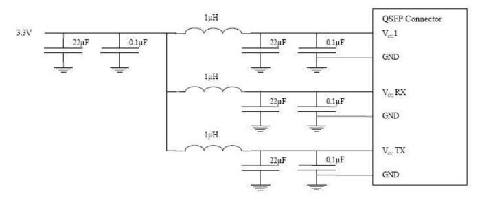
Figure 3. Host Board Power Supply Filtering
