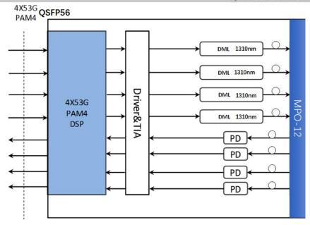
Figure 1. Module Block Diagram
