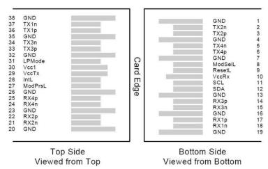
Figure 2. Electrical Pin-out Details
