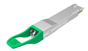
The module incorporates 4 independent channels on CWDM4 1271/1291/1311/1331nm center wavelength, operating at 100G per channel. The transmitter path incorporates 4 independent EML drivers and EML lasers together with an optical multiplexer. On the receiver path, an optical demultiplexer is coupled to a 4-channel photodiode array.
