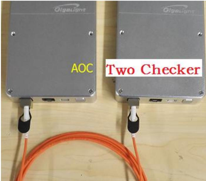
**Note:** One end module of AOC & DAC connected to one port of one checker, another end module connected to one port of another checker.
