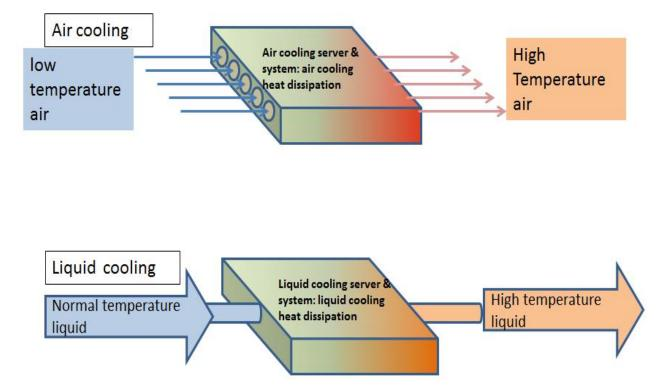
As the requirement of data traffic keeping growth and the heat flux emitted by datacenter internal chips increases constantly, traditional air cooling methods are under pressure. Liquid cooling technologies removes the heat more efficiently with dielectric fluids that have high heat capacity to improve the efficiency of energy in datacenter.
