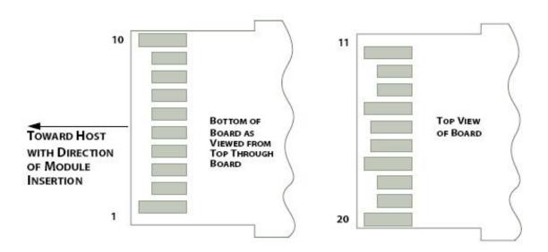
**Figure 2: Module Contact Assignment**
