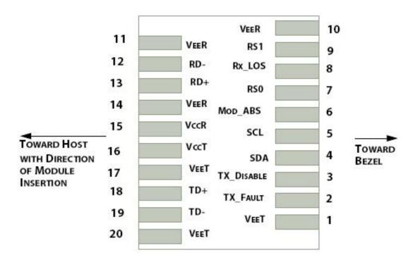
Figure 1: Interface to Host PCB
