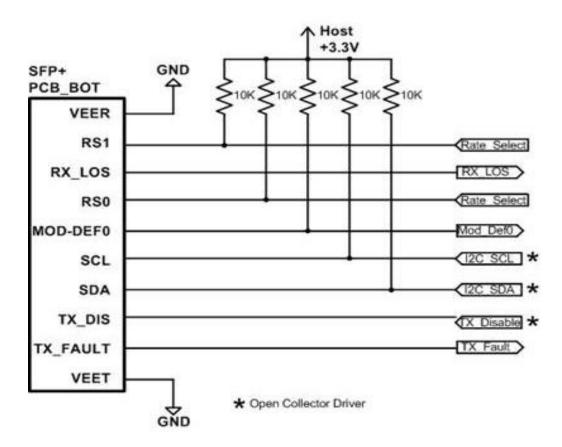
Figure3. Recommended Interface Circuit
