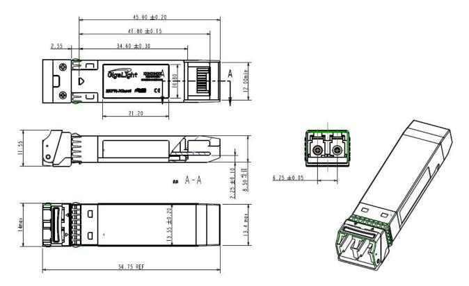
Figure4. Mechanical Specifications
